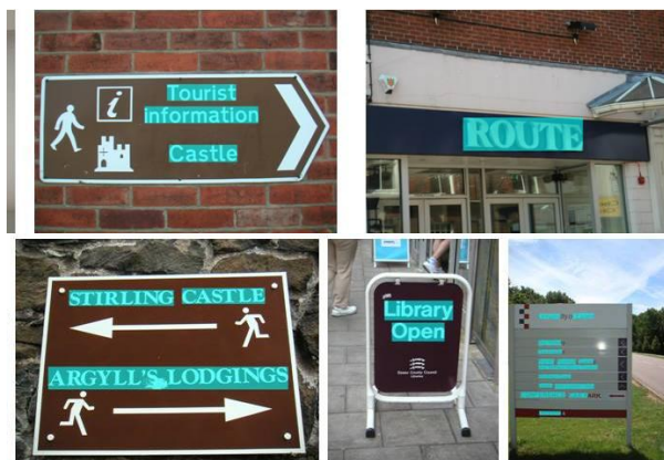
Fig. 14. Some example results of text localization on the ICDAR-2003 robust reading dataset, and the localized text regions are marked in blue. It shows that our algorithm can localize multiple text labels in indoor and outdoor environments.
