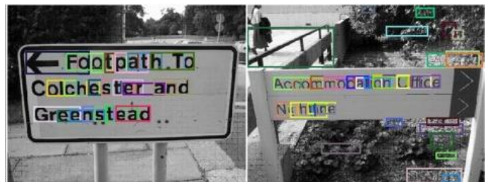
Fig. 11. Adjacent characters are grouped to obtain fragments of text strings, where each fragment is marked by a colored rectangle. The extracted image patches will be processed and input into text classifier.
