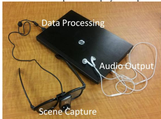
Fig. 3. A snapshot of our demo system, including three functional components for scene capture, data processing and audio output.
